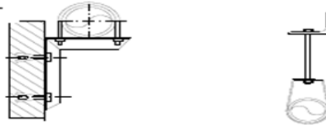
FIXED SUPPORT HORIZONTAL WALL
